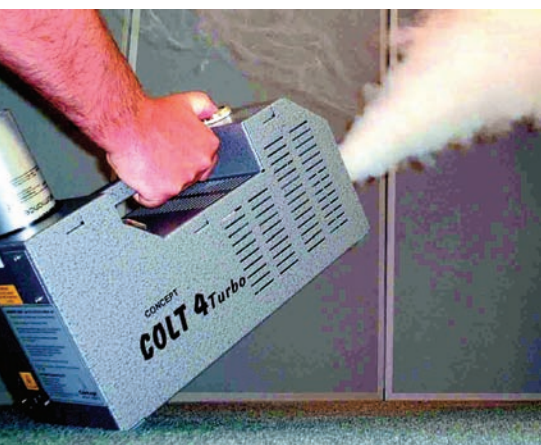
▶ A smoke generator suitable for testing air leakage from a domestic dwelling.
