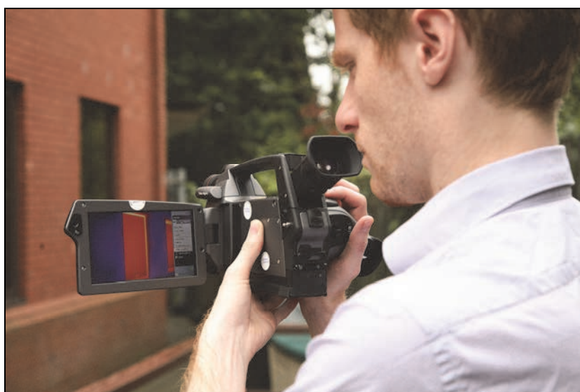
Figure 12: Thermal imaging camera in use
